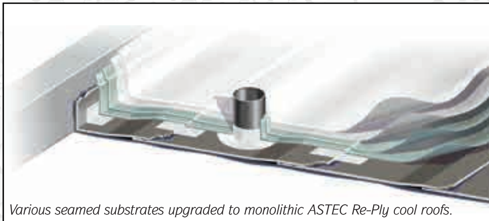
Aging metal converted to sustainable ASTEC Re-Ply cool roofing.
